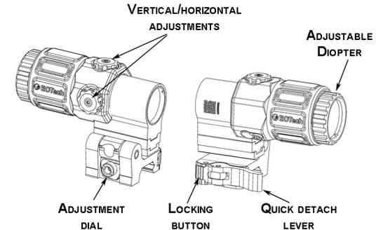
ADJUSTMENT DIAL, LOCKING BUTTON, QUICK DETACH LEVER, ADJUSTABLE DIOPTER
