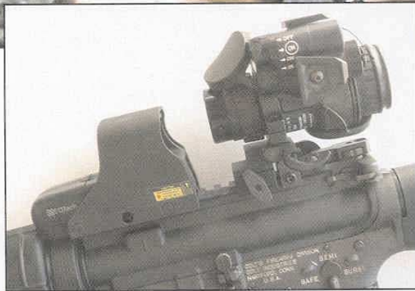
(top, inset) The M3 Tactical Illuminator weighs only 3.3 ounces with batteries. Yet, using a tungsten halogen, xenon-filled bulb and two standard DL 123A 3-volt lithium batteries, the unit delivers an amazing 80-90 lumens of white light. Shown here attached to an M16A2 by means of a GG&G mount. (left) Right now, the hottest optical sight combination available for the tactical M16/AR-15 series may very well be the new EOTech Model 500 Holographic Diffraction Sight with a Litton M983 night vision scope mounted to the rear.
